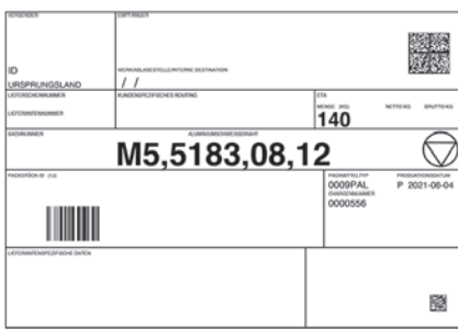
Datamatrix code code on VDA label for batch number, weight, production date and item number
