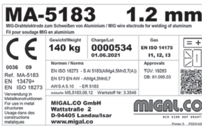
QR code on wire label for batch number, weight, production date and item number
