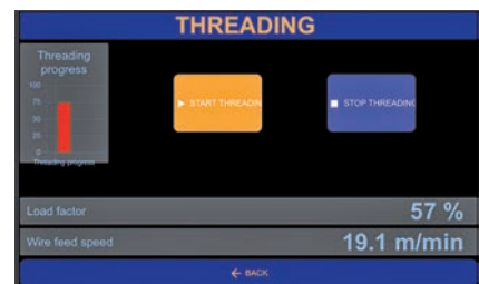
Screen for threading function - feeds the wire into the liner with a preset length
