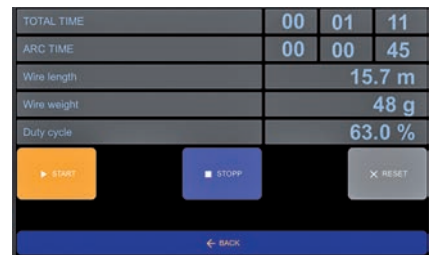
Stopwatch function for wire consumption and duty cycle
