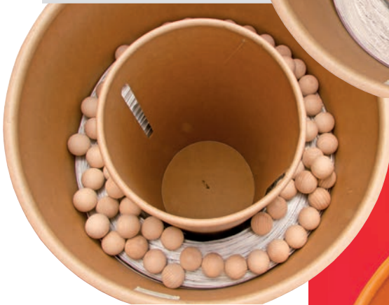
3. Eco-drum with 70 wooden balls à 40 mm diameter
