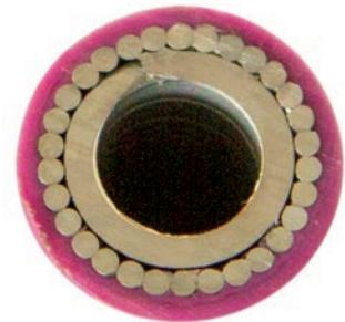
Cross section of Toughliner EXTRA
